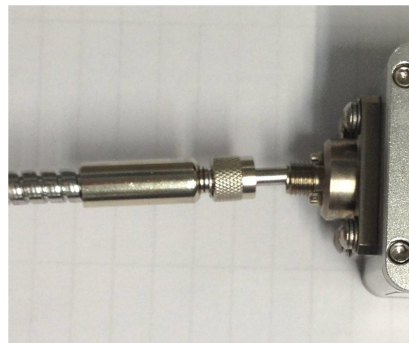
Wrong connection mode
